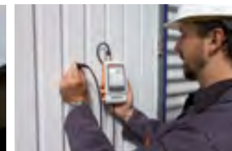
Measurement of a paint coating on steel
