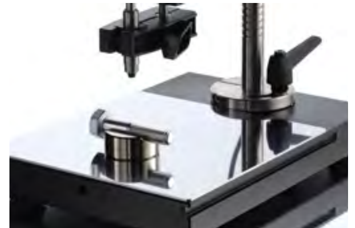
Repeatable measurement with specimen holder and probe clamped in a stand
