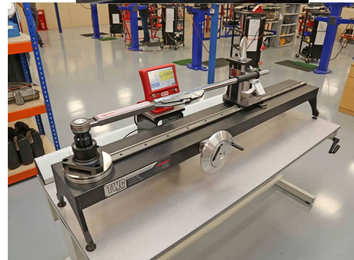
TruCheck™ 2 Plus display showing below target tolerance
