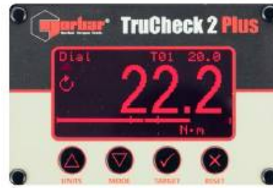
TruCheck™ 2 Plus display showing above target tolerance
