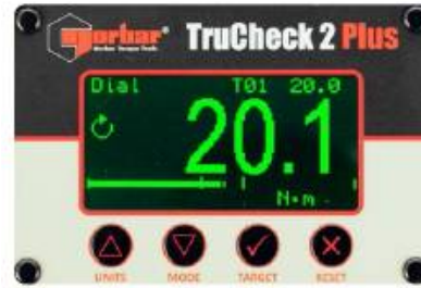
TruCheck™ 2 Plus display showing within target tolerance
